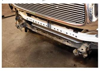
**STEP 4**Remove tow hooks from both sides.
