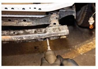
**STEP 3**Remove frame extensions and skid plate mount combo. (2001-2004 models only)
