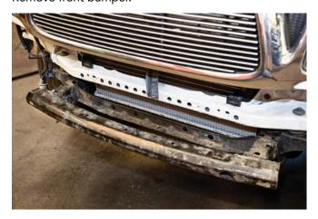
**STEP 2**Remove bumper support bar.
