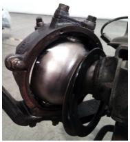
Install the one-piece split metal backing ring into the counterbore on the back of the knuckle.
